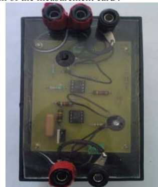
Fig 9. Solar radiation and temperature sensors
