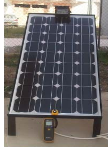
Fig.1 Photovoltaic solar SUNTECH STPO80S-12/Bb of 80W c .
